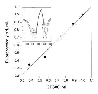
Fig. 7. Relationship between the relative fluorescence yield and the CD signal at around 680 nm for LHC II at different detergent concentrations. Inset: red region of CD spectrum of LHC II in 0.1% DM (1), 0.01% DM (2), 0.001% DM (3) and 0.0003% DM (4). LHC II was diluted in glycerol buffer media containing different amounts of DM. After 30 min the fluorescence yield of LHC II reached steady state and at this point CD spectra were recorded.
