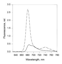
Fig. 1. 77 K fluorescence spectra of LHC II in aggregated (solid line) and trimeric (dashed line) form. Excitation wavelength was 435 nm, excitation optical bandwidth was 3.6 nm, and the emission optical bandwidth was 1.8 nm. The Chl concentration was 6  $\mu$ M and the DM concentration for trimers was 0.01% and for aggregates was 0.0003%.
