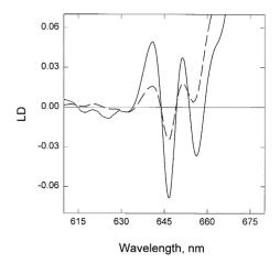
Fig. 9. 77 K LD spectrum for Chl b Qy region for the dark adapted chloroplasts containing zeaxanthin (dashed line) and after illumination to induce nonphotochemical fluorescence quenching (solid line). For the samples, O.D. = 1.
